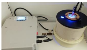
Figure 1. Photoreactor used in the experiments. LED: peak emission at 450 nm and a total power of 14.4 W.
