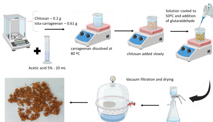
Figure 1: Scheme of the biopolymer blend production process. Source: Author.
