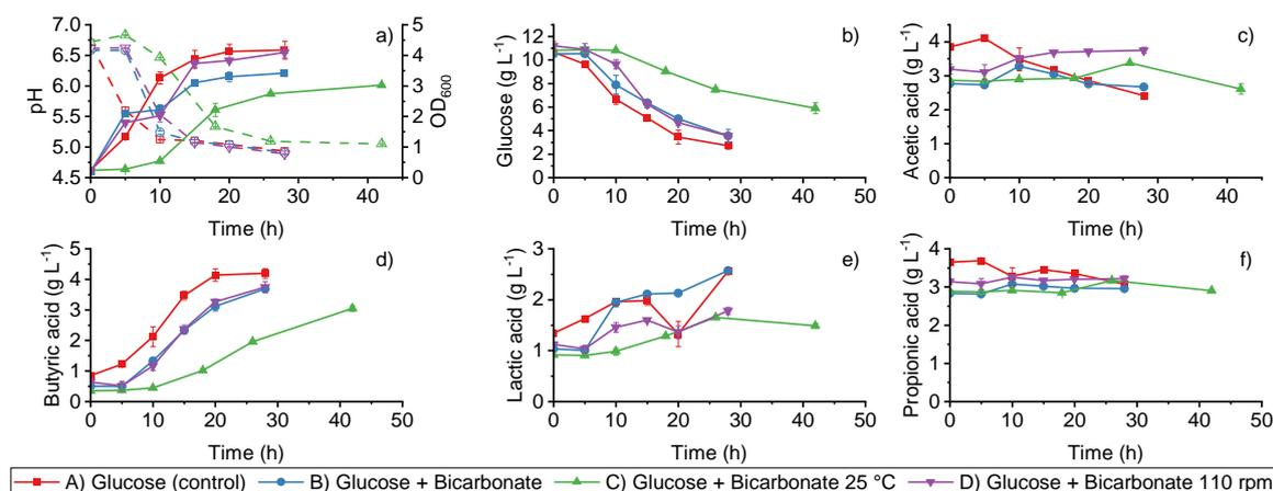
**Figure 1** Growth experiment performed with *C. beijerinckii* Br21, with addition of 10 g L<sup>-1</sup> KHCO<sub>3</sub>. Altered parameters were agitation and incubation temperature. OD<sub>600</sub> (filled symbols) and pH (empty symbols) (a), glucose (b), acetic (c), butyric (d), lactic (e), and propionic (f) acids. Error bars represent standard deviation calculated using a biological triplicate.
