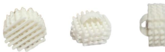
Figure 1. CAD-designed poly(lactic acid) carriers used to immobilize commercial glucoamylase..
