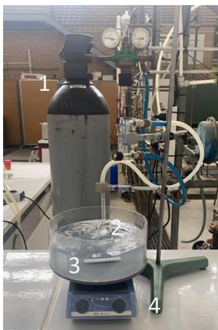
Figure 1 System for dissolved O 2 experiments composed by a gas cylinder (1), a diffusion rock (2), a cylindrical reactor (3) and a magnetic stirrer (4)
