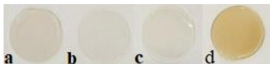
Figure 1 Films obtained by the casting method: a) Pectin b) Inulin, c) \beta -Glucan and d) RSF
